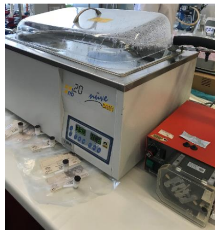
Figure 3.6 - Water bath for heating system
