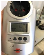
Figure 3.9 - Energy measuring device PM 231
