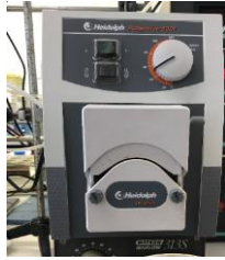
Figure 3.1 - Pumping system and peristaltic pump for acidification
