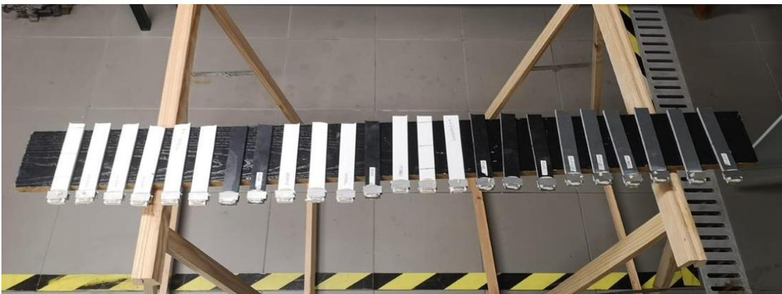
Figura 66 - Provetes com as dobradiças piano coladas
