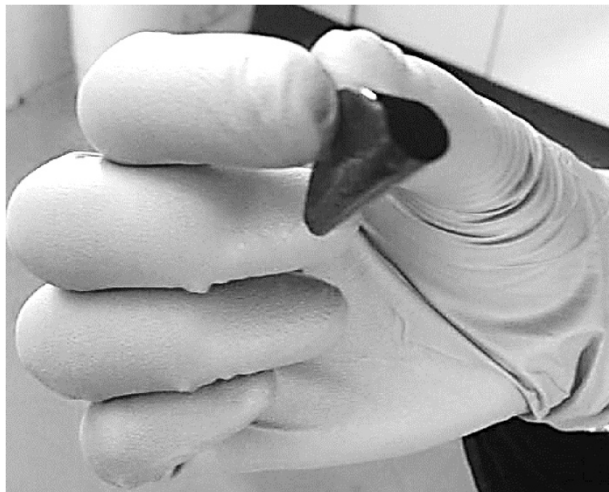
Figure S.5. Illustrative figure of the flexibility of the prepared carbon membranes; sample CMSM 550.
