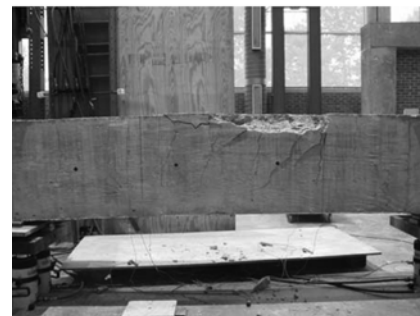
(b) Specimens with splices confined by transverse reinforcement
