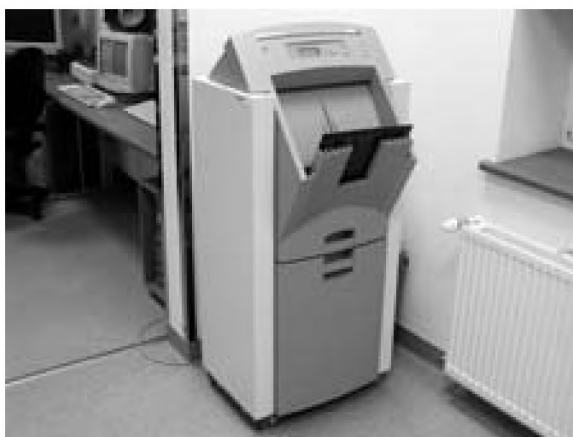
Figure 12. Thermal printer: Agfa DryStar 3000.
