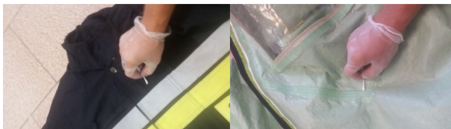
Figure 2. An example of sample collection from special NOMEX clothing (on the left ) and type 1a heavy gas-tight clothing (on the right side).
