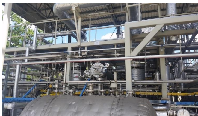
Figure 6. Photo of a fragment of the liquefaction system of post-cracking products and one of the intermediate tanks.
