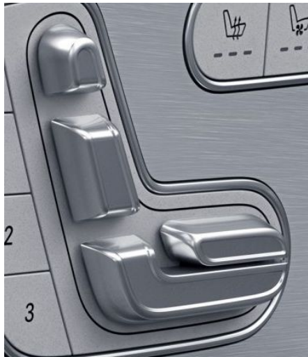
Figure 5.3: Example of a natural mapping for the controls allowing to adjust a car seat.
