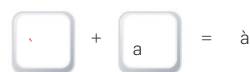
(d) Diacritics work as dead keys: visible output is produced upon subsequent input of a letter.
