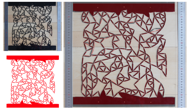
Figure 10: Matching of simulation and physical realization. Network (same as in teaser) extended in the vertical direction with a strain of 6%. Physical realization (top left), simulation (bottom left), superimposed physical realization and simulation (right)
