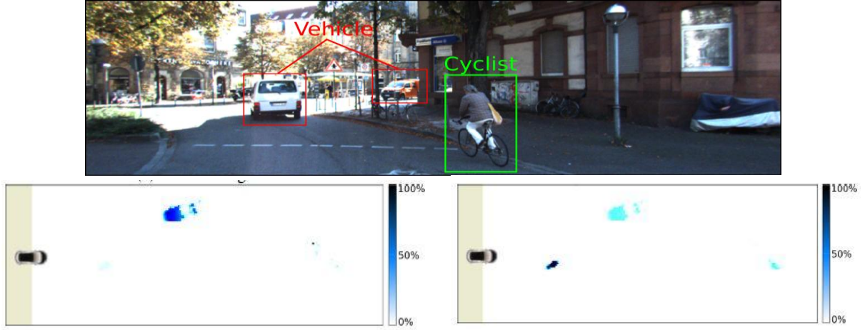
Figure 12: Probability of Collision with Injury Risk (PCIR) approach, evaluated using KITTI dataset – Top: Scenario analyzed with a classification of moving entities – Bottom left: Results from the VRU perspective – Bottom right: Results for the Economical/political perspective.
