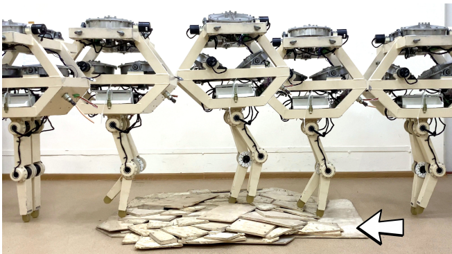
Fig. 4: The robot is able to walk "blindfolded" over small obstacles; no any kind of vision/remote sensing is used. Refer to Fig. 5 for a plot of the signals for this experiment.
