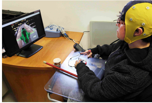
Figure 3. Experimental setup of the MI-BCI system. The pilot is wearing the EEG cap and EMG electrodes are placed on her hands.
