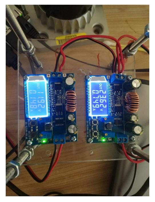
Fig. 3.8. The DC-DC Buck Boost converter displays showing the voltages being supplied to the LIDAR and the Carrier Board. The system is housed inside the metallic box on top of which the LIDAR is fitted.
