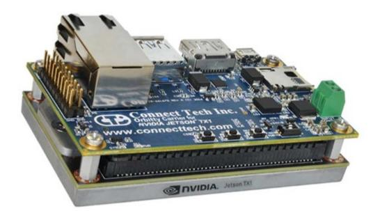
Fig. 3.7. Nvidia Jetson Tx2 System on Chip Source with the Carrier Board
