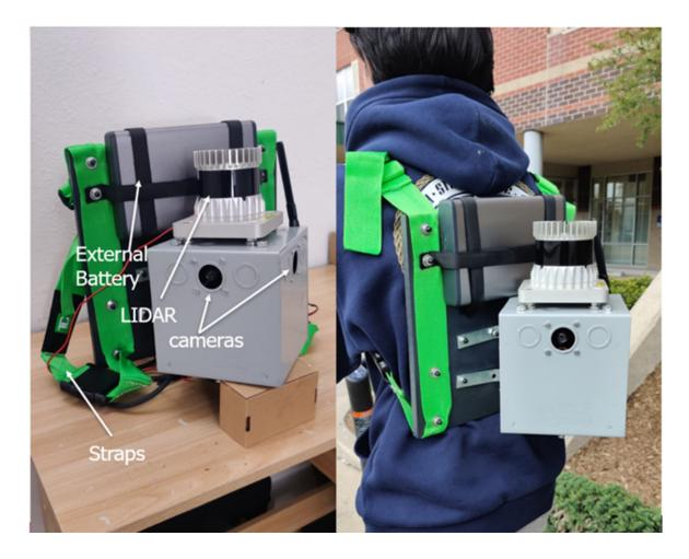
Fig. 3.2. The Data Acquisition System
