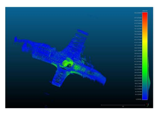
Fig. 6.10. 3D mapping (.ply file) of the Stutz lab viewed using ccviewer from collected data
