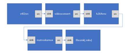
Fig. 3.14. G-streamer Non Hardware Accelerated video recording pipeline
