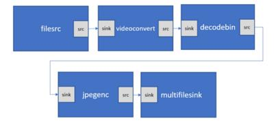
Fig. 5.8. Gstreamer Pipeline for converting captured image frames into a single video.
