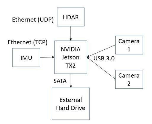
Fig. 3.12. Basic Data flow for the system
