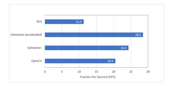
Fig. 6.4. Frame rate comparison for 2x Logitech c920 cameras over USB 3.0 utilizing different recording methods
