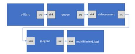
Fig. 3.16. Gstreamer Non Hardware accelerated frame storing pipeline
