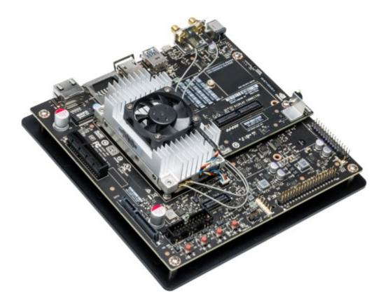
Fig. 3.6. Nvidia Jetson Tx2 Development Board with SOC
