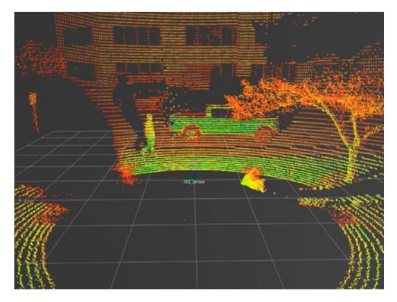
Fig. 3.11. Rosbag LIDAR data visualization using Rviz
