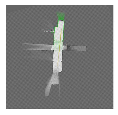
Fig. 6.9. 2D Probability grid showing the map of stutz lab(white and grey) and vehicle trajectory(Yellow line) in the Stutz Lab from collected data
