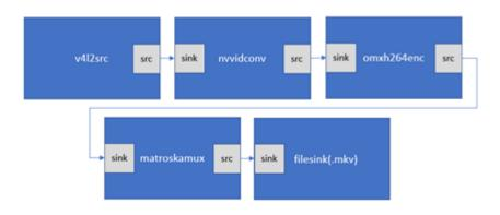
Fig. 3.15. G-Streamer Hardware accelerated video recording pipeline
