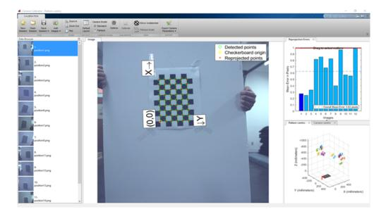
Fig. 4.2. Intrinsic Matrix calibration using MATLAB Camera Calibrator
