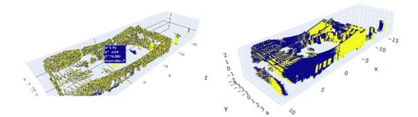
Fig. 5.2. 2 Degree yaw difference induced in the point cloud due to the difference in UDP packet decoding methods. Left Image shows the same point cloud processing method (yellow and blue mixed) and Right image shows difference due to difference in math library and Trigonometric Table based processing
