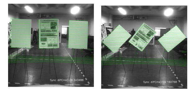
Fig. 4.4. Fusion Overlay on 3 poster boards using collected LIDAR and camera data
