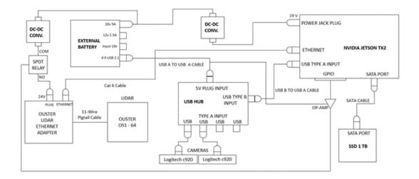
Fig. 3.9. Collection System Architecture
