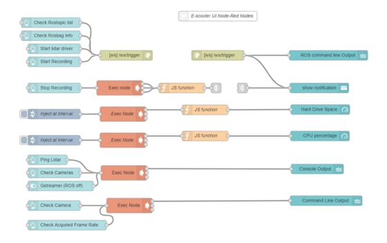
Fig. 3.20. Node-Red Programming Flows for UI
