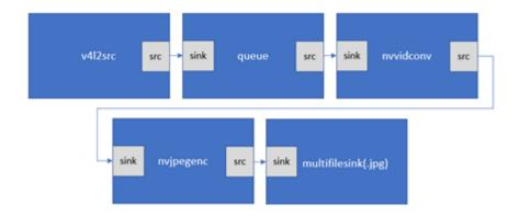
Fig. 3.17. Gstreamer Hardware accelerated frame storing pipeline
