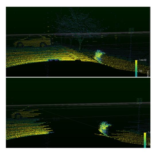
Fig. 6.1. Visualization of Packet Loss in a frame in the dark area (below) compared to no packet loss in a frame (above)
