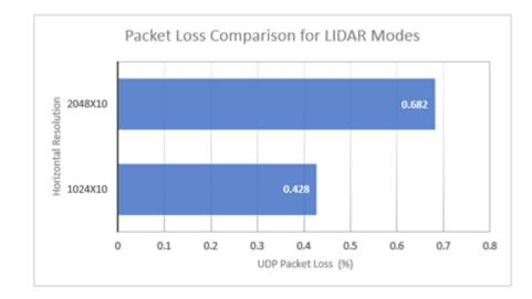
Fig. 6.2. Percentage Packet Loss Comparison for two LIDAR modes
