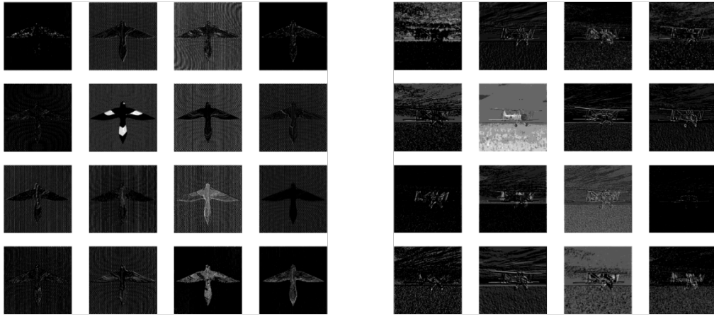
Fig. 2.12.: RGB* output of layer res2c_out in the ResNet-101 backbone showing the first sixteen 256x256 layers from the 256x256x256 tensor. Left: Kite. Right: Plane.
