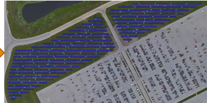
Figure 5. Final proposed PV power plant layout located on the north sector of CIRA's long term parking facility
