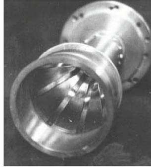
**Abb. C.6** Anodenblock eines relativistischen Magnetron mit axialer Auskopplung. (© 2010 IEEE. Reprinted, with permission, from J. Benford, History and future of the relativistic magnetron, 2010 Int. Conf. on the Origins and Evolution of the Cavity Magnetron, p. 44, April 2010 [113].)
