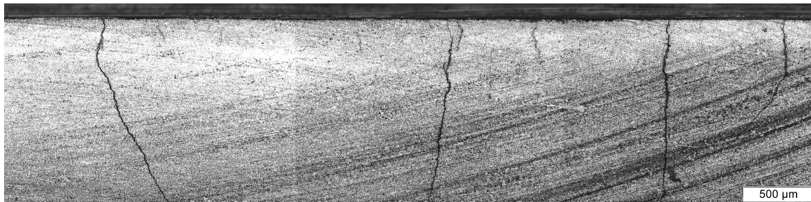
Figure 10. Stitched image of the specimen edge after n = 10^6 cycles for R = \infty . The total length of the image is about 5.7 mm. The top 0^\circ -layer is separated along the whole image length and beyond by delamination.
