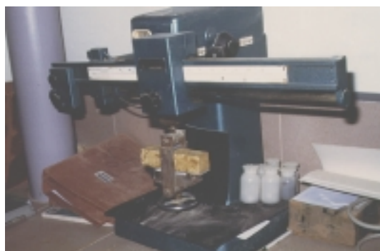
Figure 5: Prismatic specimens flexural test
