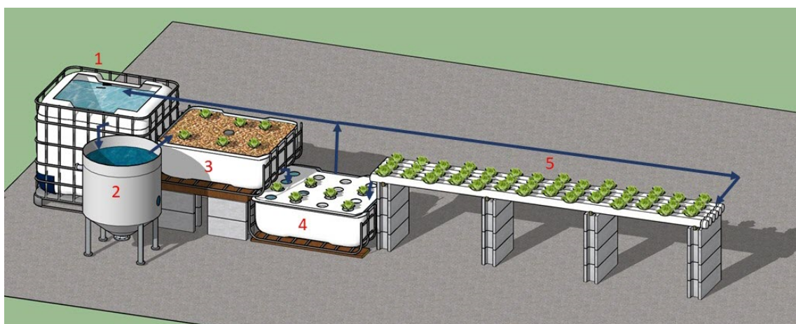
Figure A1. Schematics of the SAS: (1) fish tank; (2) clarifier; (3) biofilter and media bed; (4) sump and floating raft; (5) NFT. Blue arrows represent the direction of the water flows.
