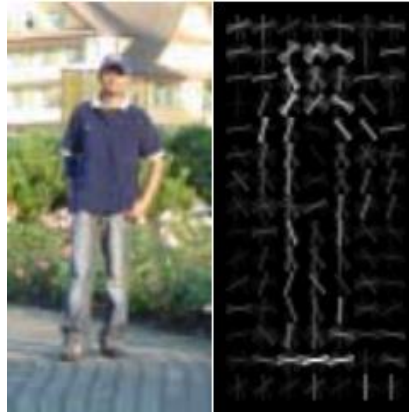
Figure 20 - HOG detectors cue mainly on silhouette contours [36]. Human body feature representation is depicted.
