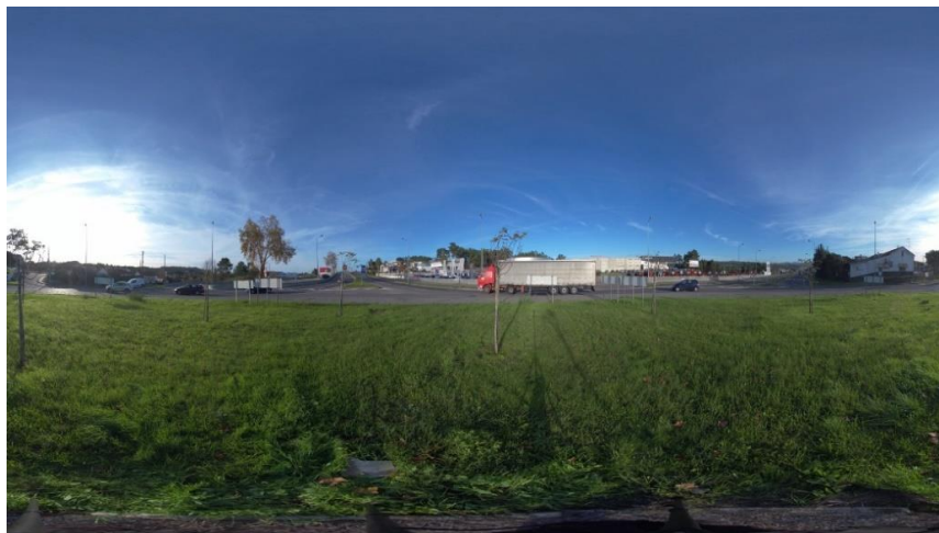
Figure 14 - Example of a 360° video frame projected onto a 2D plane with ERP approach.
