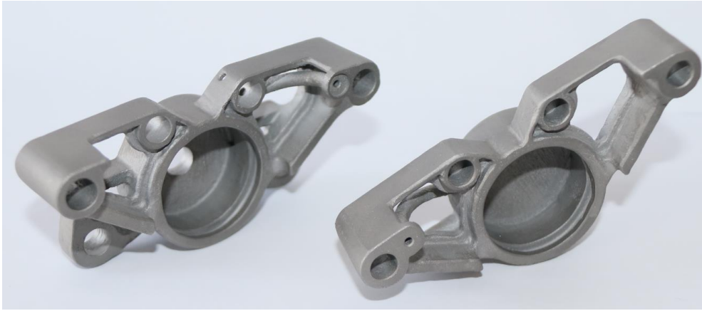
Figure 6.5- Prototype 3, H13 Steel, after sand blasting.
