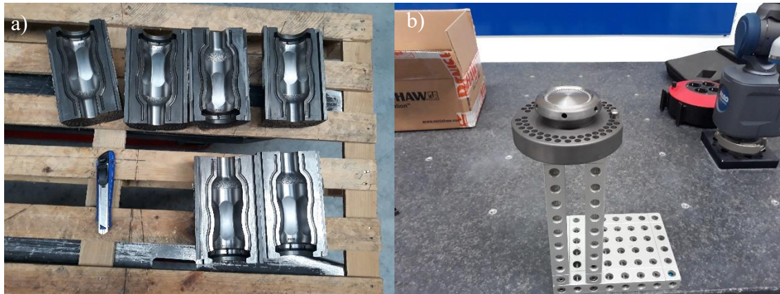
Figure 48 – Set of cast iron moulds: a) Cast iron mould halves; b) Cast iron mould bottom
