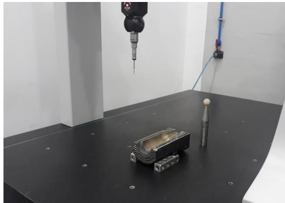
Figure 70 - Mould fixed on the CMM
