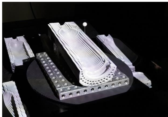
Figure 60 - Polished cast iron mould being scanned by structured light
