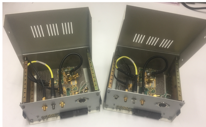
Figure 33: The complete 27 GHz RF Frontend using X-Microwave Innovative Modular Building Block System.
