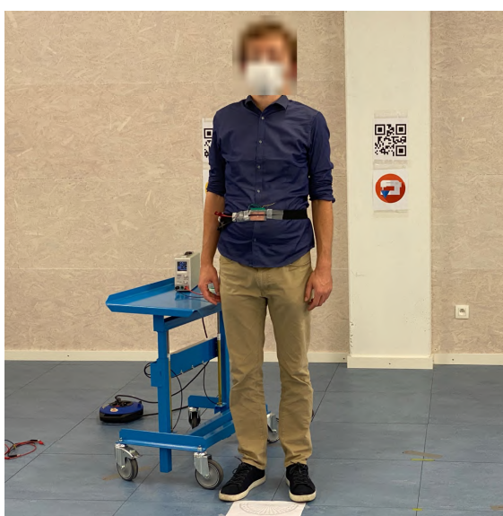
(a) Test subject fitted with the belt hosting the sensor node. This is the on-body deployment position for \phi = 0^\circ . The system is powered by an external power source for measurement purposes.
