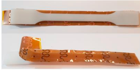
Figure 1: Over-molded sample (top), Trimmed peeling test sample (bottom)
