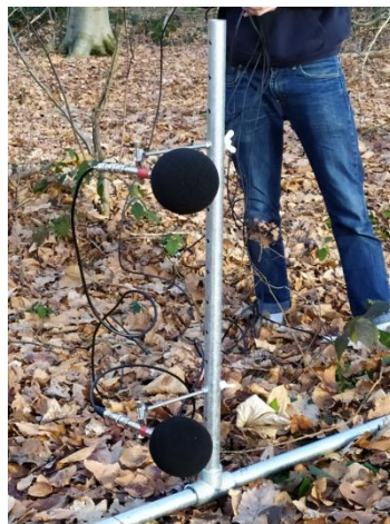
Figure 1: Experimental set-up showing the two microphones for the level difference measurements.
