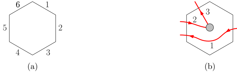
Figure 7.4: (a) Labeling of the edges of a hexagonal tile in a clockwise direction. (b) Example of a configuration of lines running through tile 10 in Fig. 7.3(a) (when counting from left to right and from top to bottom). Each line segment is assigned a unique integer label.
