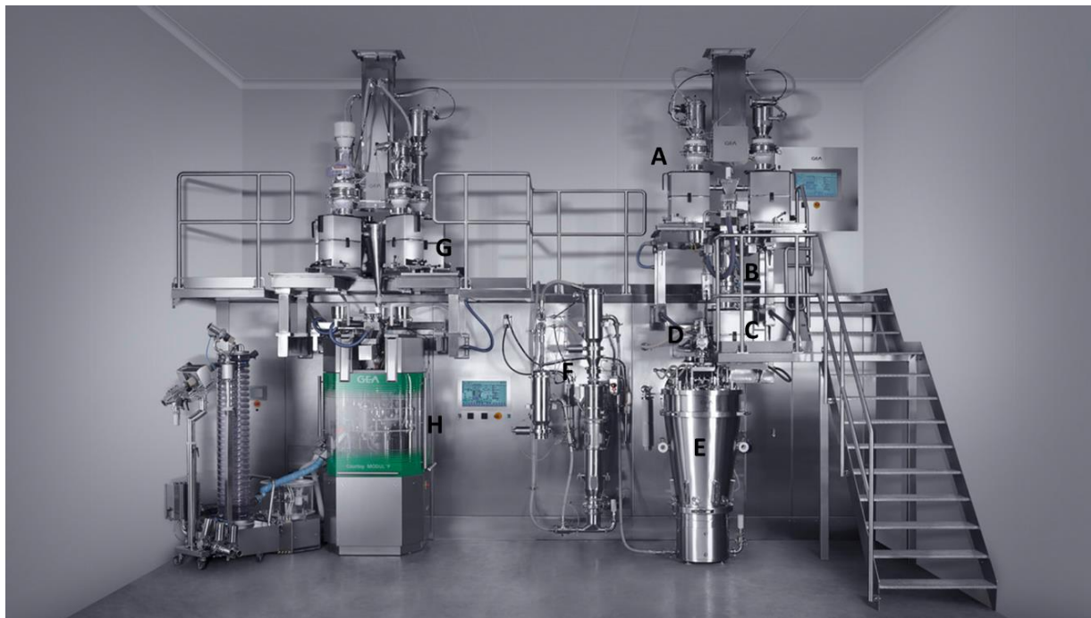
Figure 1.6: ConsiGma™-25 continuous tableting line with (A) several loss-in-weight feeders, (B) a continuous powder blender, (C) a loss-in-weight feeder to dose the powder mixture, (D) a twin-screw wet granulation unit, (E) the six-segmented fluid bed dryer, (F) the granule conditioning unit with integrated mill, (G) loss-in-weight feeders and a blender to mix the external phase with the milled granules and (H) a Modul™P tablet press (Courtesy of GEA Pharma Systems).
