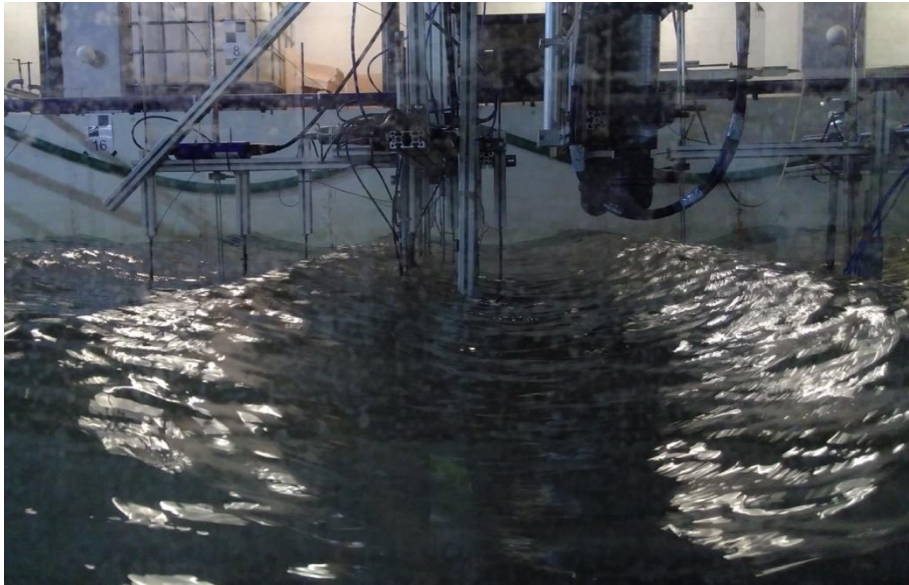
Figure 4 Sideview of waves passing over the mound during testing (May 10) The mound is positioned below the vertical aluminum bar.
