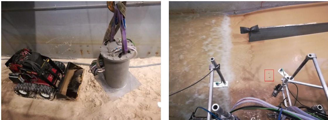
Figure 47: CCM+ instrumentation. Left photo: Moving CCM+ tank 2. Right photo: Probes of CCM+ tank 1 (in red square) measuring within the bed.
