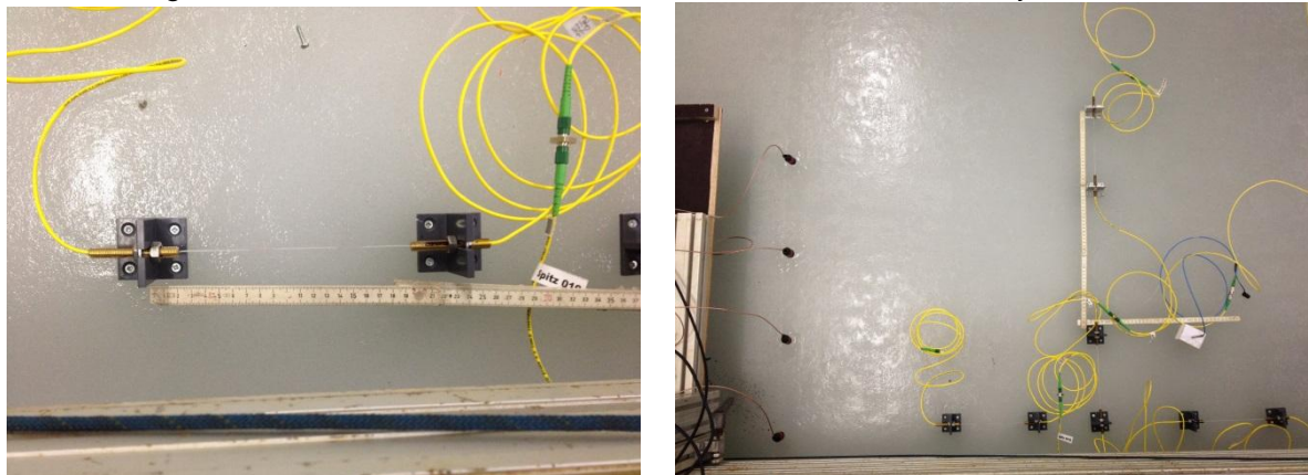
Figure 4. Scheme of the installation of FBG sensors on the ice by x < 20 m.
