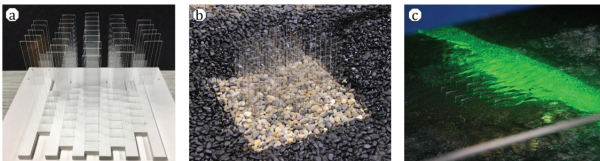
Figure 1. Design of the artificial patch (a), meeting the allometric characteristics of a natural willow plant, installed in the flume (b), and during experiments (c).
