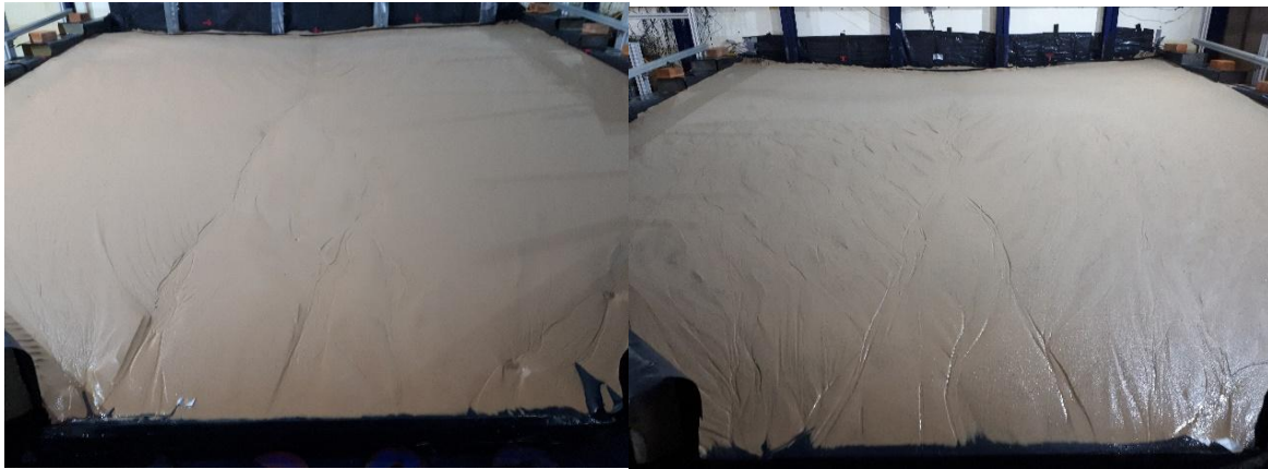
Figure 6. Typical erosion pattern for plot 1 with fine sand (left) and plot 2 with medium sand (right).
