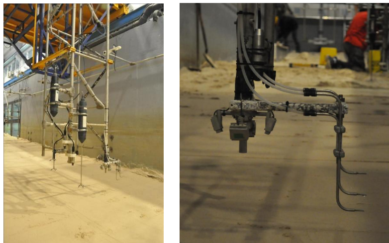
Figure 5: Instrumentation on the mobile frame. Left photo: mobile frame. Right photo: ACVP and the three nozzles of the TSS.
