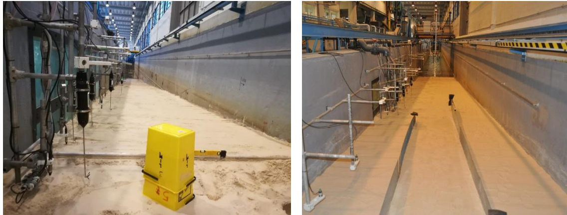
Figure 15: Preparation of the beach profile (view towards the wave paddle). Left photo: manually shaped beach. Right photo: filling the wave flume (dividers in the front).
