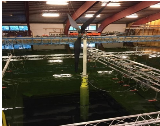
Figure 1. Impression of the scaled spar-buoy wind turbine layout used during the Hydralab+ tests.
