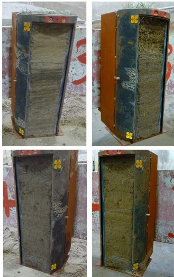
Figure 6: Impressions of the vertical soil core faces before (left) and after (right). Top: sandy sediment from Warton (right); Bottom: clay-rich sediment from Tillingham (replicate 2 prior to exposure (left) and after exposure to conditions 5-8 (right)) (nb: structures from the slicing clearly visible in both)
