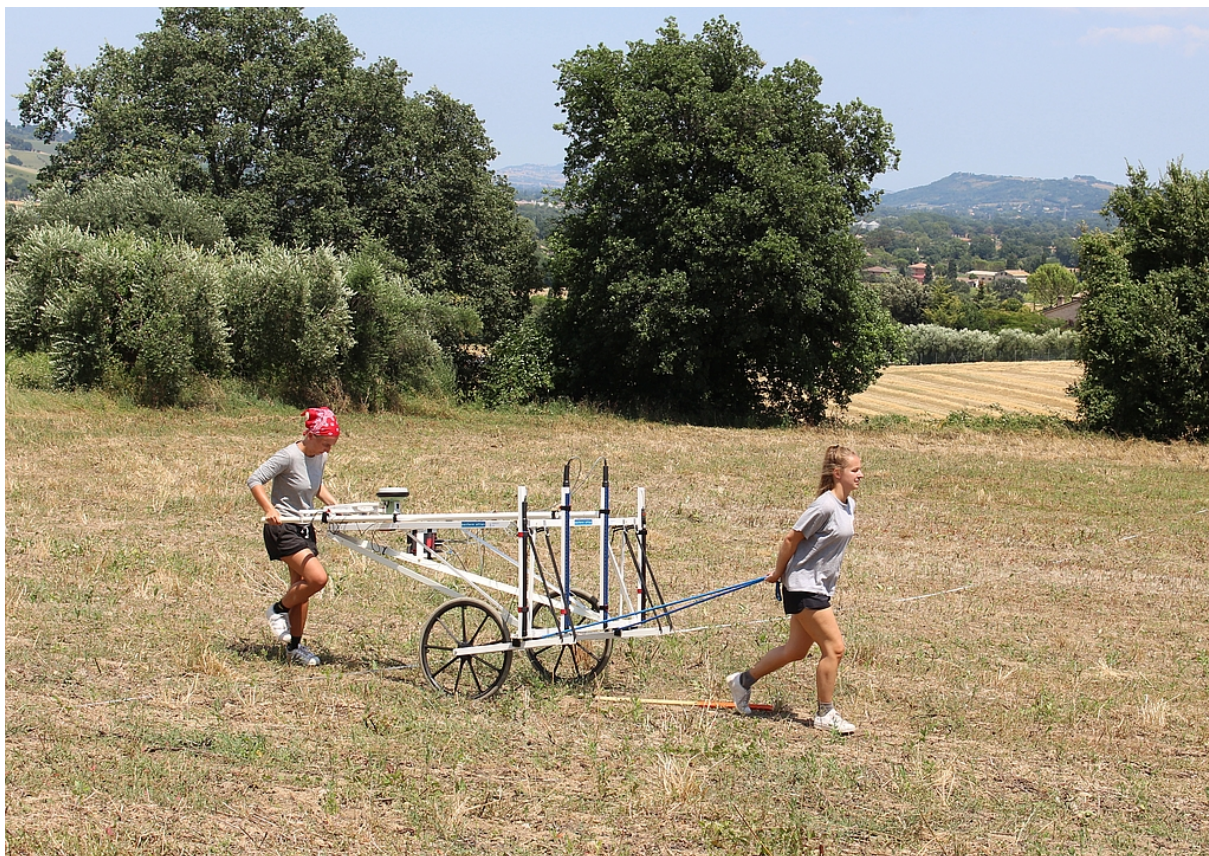
Fig. 3. Magnetic gradiometry survey at Monte Franco in 2018.
