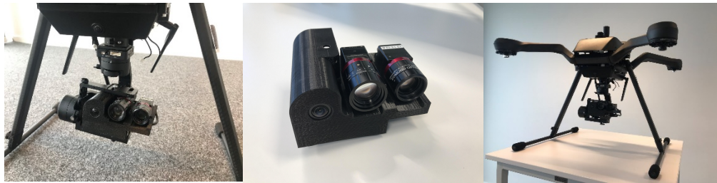
Figure 1: Prototype hyperspectral payload on Airobot Mapper.
