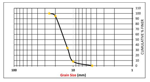
Figure 2. Coarse aggregate sieve analysis.
