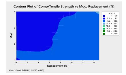
RHAC. The contour plot among the tensile/flexural strength ratio is shown in Figure 8 below.
