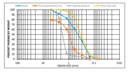
Figure 1. Fine aggregate sieve analysis.
