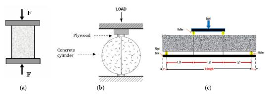
Figure 3. Strength testing machine mechanism (a) compressive, (b) tensile, (c) flexural tests.
