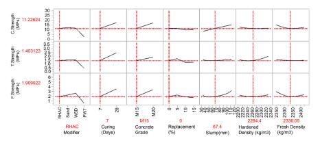
Figure 6. Prediction profile graph for the analysis of mechanical properties of green concrete.
