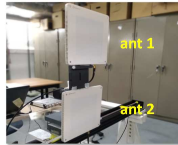
Fig. 17. Two vertical antennas deployment for SARFID and Tagoram.
