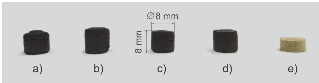
Figure 1. Schematic diagram of mixed fuel pellets preparation: a) lignite pellet, b) pellet with 10% sawdust, c) pellet with 25% sawdust, d) pellet with 50% sawdust, e) homogeneous sawdust pellet.
