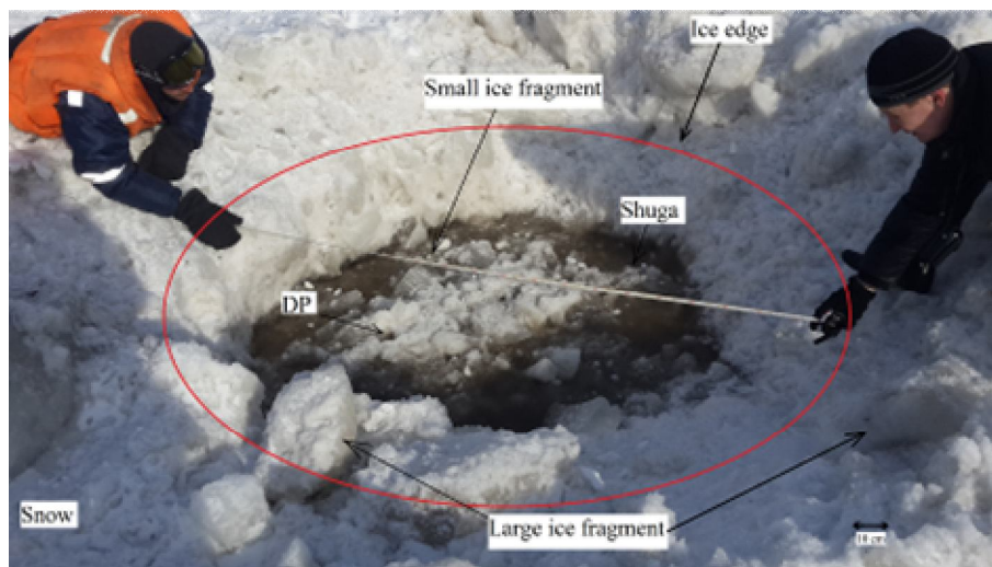
Figure 1. Lane in snow-covered ice cover. Full-scale test 2017. Bar represent 10 cm. Photo by S. Kul'kov
