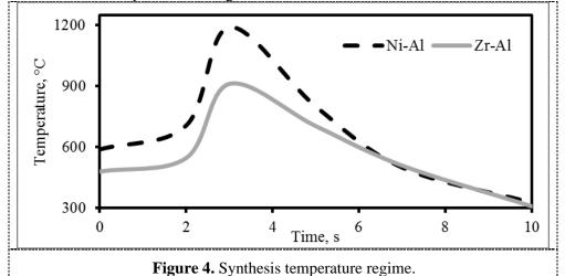
The maximum matrix synthesis temperature for a system of Ni-Al is equal to 1200 °C. A system of Zr-Al has lower thermal effect with the maximum temperature of 900 °C.
