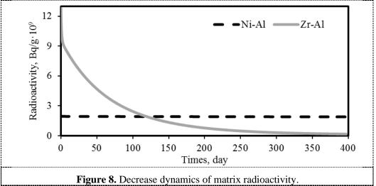
It can be observed that Ni-Al matrix radioactivity decreases slightly during one year. This fact is stipulated for a high quantity accumulation of Ni<sup>63</sup> isotope having the half-life of 100.1 years in the sample.
