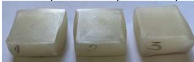
Figure 5. Samples made of PLA plastic 3D printed using fused deposition modeling after compression tests.
