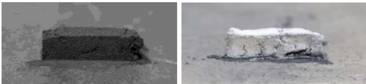
Figure 2. The typical views of aluminum nanopowder cuboid samples before combustion and after.
