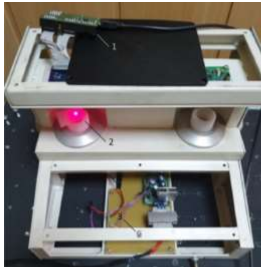
Figure 2. Experimental setup: 1 – developed module, which consist of camera and microcontroller, 2 – control plasma in a cuvette on the sample table and a solid-state laser, 3 – laser driver.
