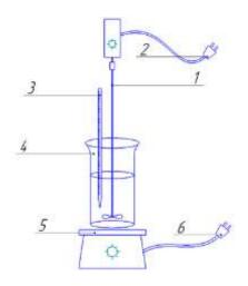
Figure 1. Simplified diagram of the laboratory unit for the transesterification reaction:1 automatic blade stirrer: \_ 2 – power-intake connection yoke for blade stirrer the electricity to mains; 3 – thermometer; 4 – heat-resistant beaker; 5 – electric stove with heat control; 6 – power-intake connection yoke for electric stove to the electricity mains.
