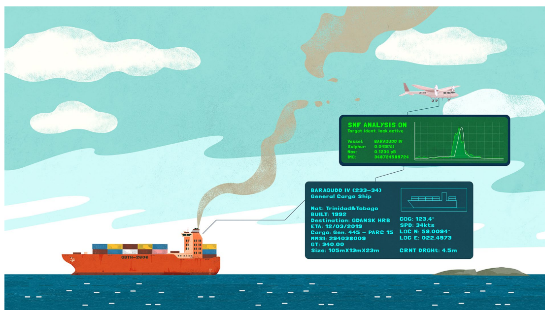
Figure 4. Airborne monitoring of FSC and NO x in ship exhaust. The ratio of SO 2 and CO 2 and NO x and CO 2 , respectively, is used to deduce the emission factor from the ship. A similar approach is illustrated on the front page for fixed measurements.
