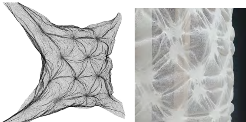
Figure 4: Comparison between a simulation made with the processing program and a textile, with the same repeated geometric (chesterfield) pattern, in wind.
