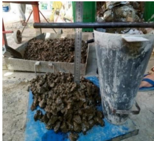
Figure 7. Slump measurement of fresh concrete.
