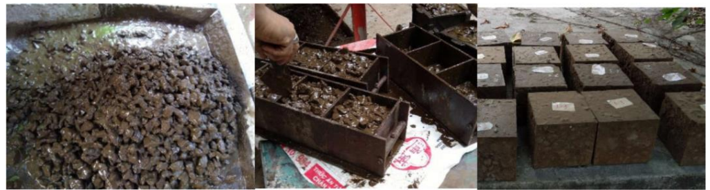
Figure 5. Manufacturing procedure of geopolymer recycled aggregate concrete (GRAC) specimens.
