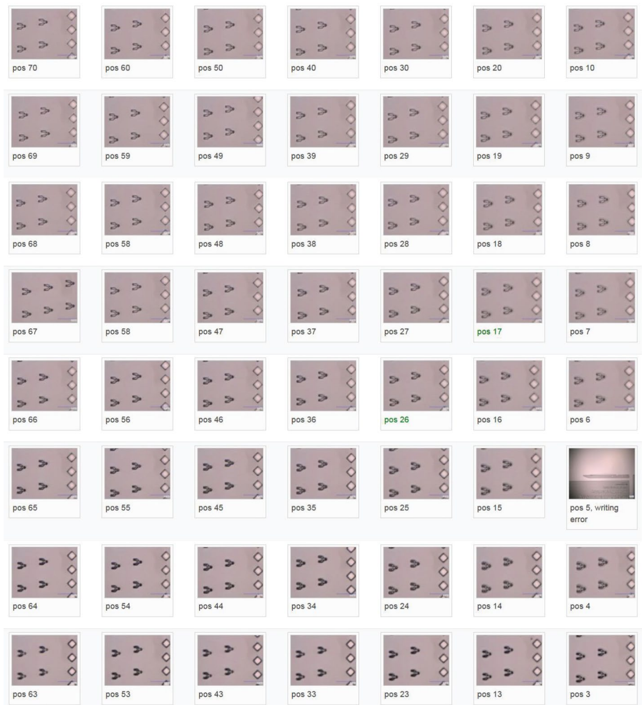
Figure S3. Light-microscopic inspection of the test array from Fig.S2. For all positions, images were taken from the same part of the test structure at constant microscopic settings. This overview is best suited to narrow down the parameter space to useful values. Close-ups indicating the subsequent decision making process are shown in Fig.S4
