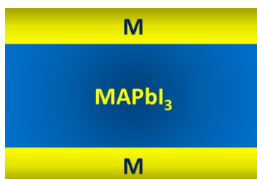
Figure 2.5. Schematic of a M/MAPbI 3 /M parallel plate capacitor.
