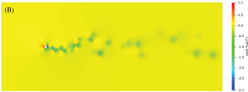
FIGURE E2 Instant snapshot of the normalized velocity for a two-dimensional flow over cylinder at Re = 3900 at t = 50 s [Color figure can be viewed at wileyonlinelibrary.com ]
