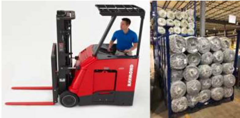
Figure 15: Standing Forklift Example [v] and Stackable Pallet Rack Storage Example [vi]
