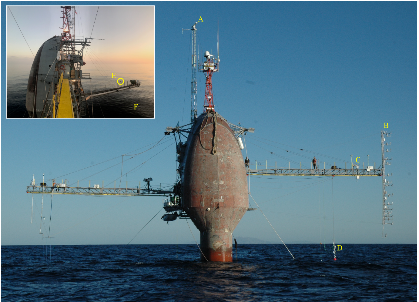
Fig. 2: View of FLIP during CASPER-West. (Background) A view from the keel-side with (A) the marine radar used for NIW detections; (B) ASIM mast on portside boom; (C) radiometric sea surface temperature sensors; and (D) FLIP 's lowest observing platform (FLOP), a surface-following meteorological mast buoy. Inset: (E) location of field camera used for surface visualization, the field of view was centered on the ASIM mast and (F) location of temperature string tether to the face boom. ADCP's were mounted on the face-side, along the spar on a frame \sim 15 m below the surface and that extended out a few meters from the hull.
