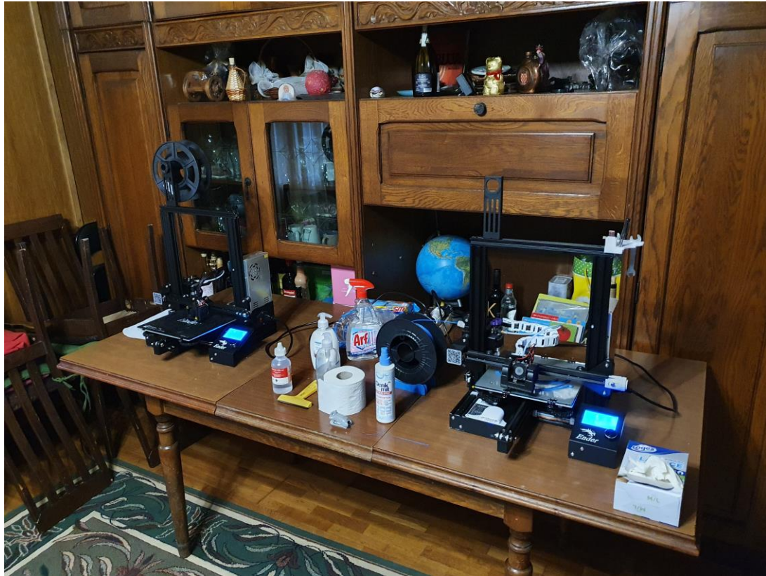
Figure 2. 3D printing of face shield parts in homemade production settings (Prusa Face Shield).
